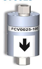
The unique design of the valve is such that, provided the supply gas pressure remains constant, a consistently accurate flow of gas can be maintained when the downstream pressure changes. A typical example would be when filling a large buffer tank or a pipe work system, especially from a Nitrogen separation system.
