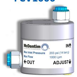
The unique design of the valve is such that, provided the supply gas pressure remains constant, a consistently accurate flow of gas can be maintained when the downstream pressure changes. A typical example would be when filling a large buffer tank or a pipe work system, especially from a Nitrogen separation system.
